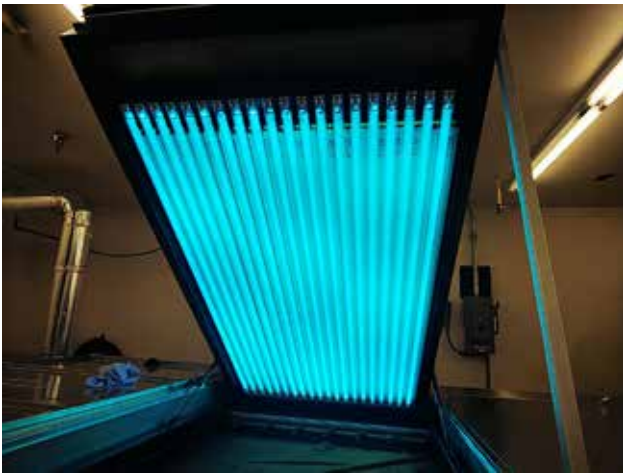
Inline-UV post-exposure ensures high plate uniformity
